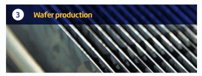
Wafering of the blocks takes place using wire saws at the Group's facility in Erfurt, Germany. Wafers are manufactured to meet the highest standards and we work with our customers to increase product quality.
